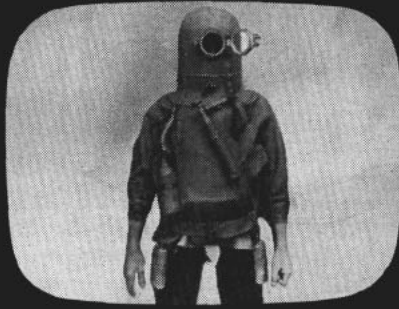
1914 SUBMARINE ESCAPE apparatus used by U.S. Navy was British Siebe-Gorman unit similar to 1819 design.
