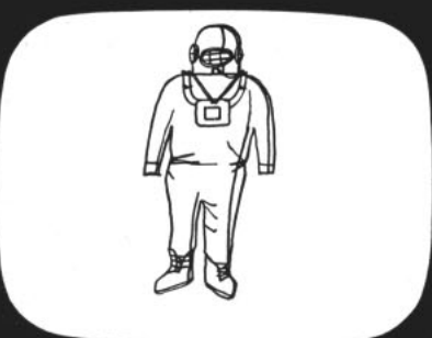
SIEBE'S "CLOSED DRESS" of 1819, waist-length "open dress," developed into the full-length suit used today.
