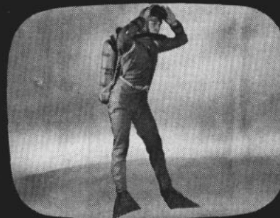
SCUBA—Self Contained Underwater Breathing Apparatus—plus rubber suit is gear for cold water longer missions.
