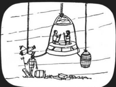
ASTRONOMER HALLEY conducted diving-bell experiments in 1690 leading to solution of breathing problems.
